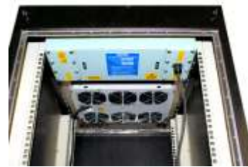
Inside I/O panel + fans
